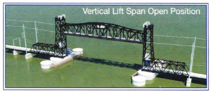
A Vertical Lift Bridge which will be similar to the one built between South Amboy and Perth Amboy. Bridge
