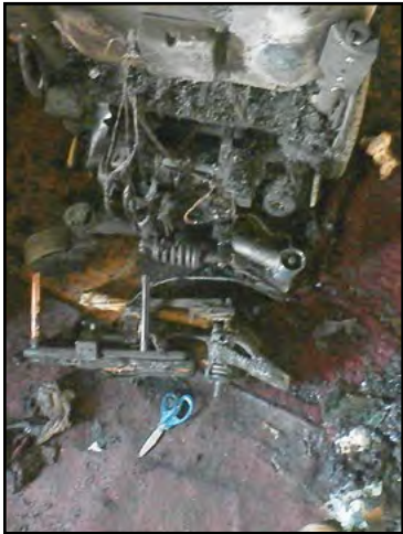
Shown above is damage to a woman's Motorized Wheelchair which is speculated to have started the fire. *Photo by Joe Bayona
